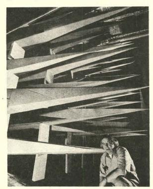
JIM REED with some of the RF absorber cones in EMES. Jim conceived the idea of a building that is essentially a coaxial transmission line.
